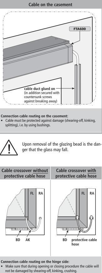
• Protect cable feedthrough in profile e.g. by using cable bushings, cable transitions.
