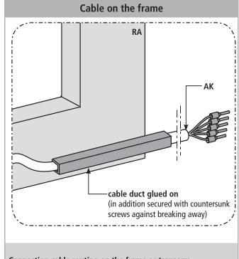
Connection cable routing on the frame or transom:
